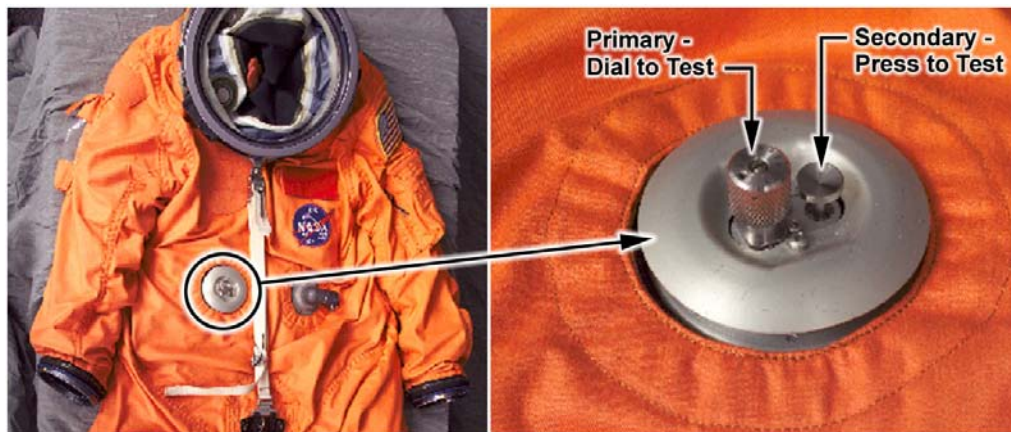
Figure 2-3. Dual suit controller
