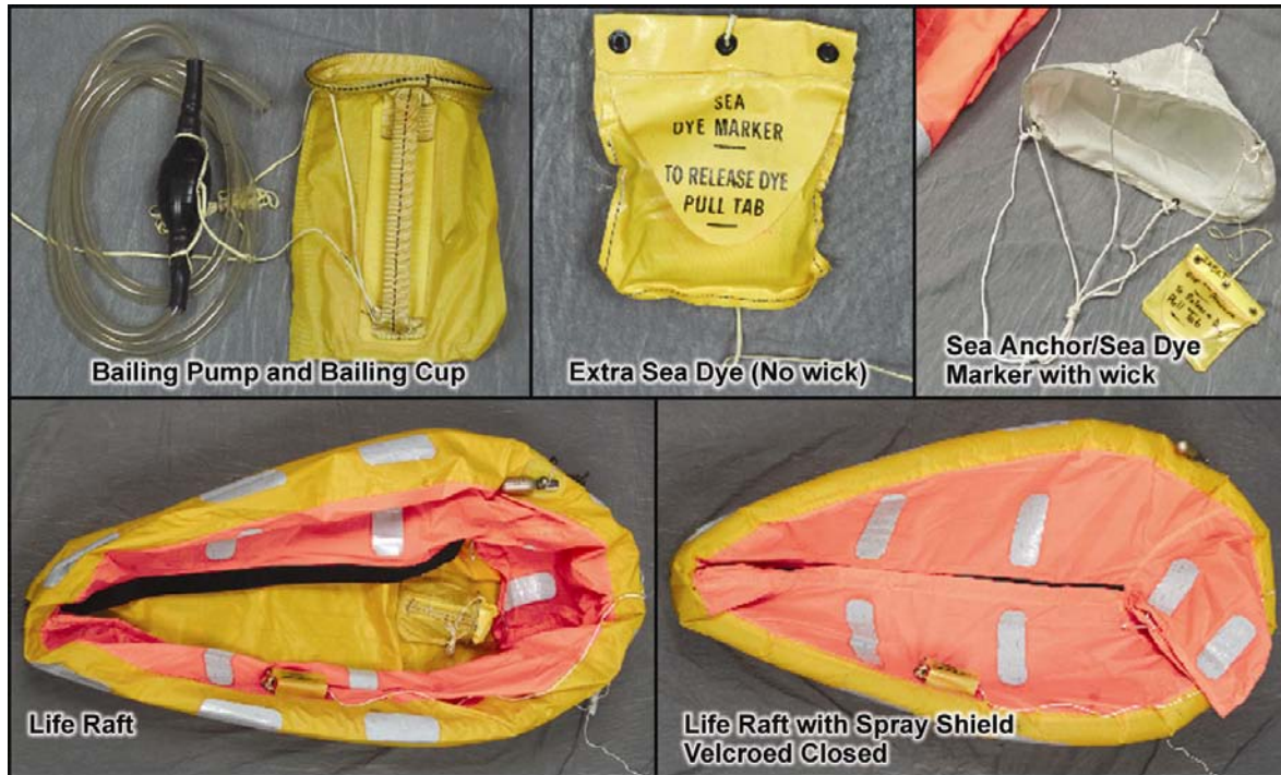
Figure 2-25. Rescue/survival gear, PPA/life raft
