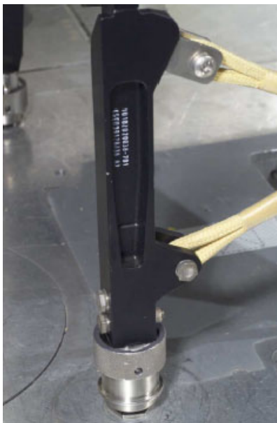
Figure 3-5. Quick disconnect fittings
