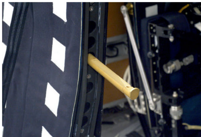
Figure 3-6. Emergency egress step
